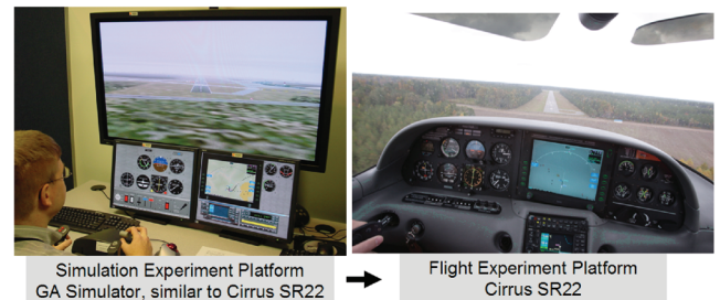
Fig. 5 HVO experiment platform progression (note commonality of HSI and MFD).
